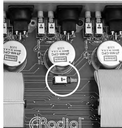
Each channel has a lift switch directly below the transformer.
